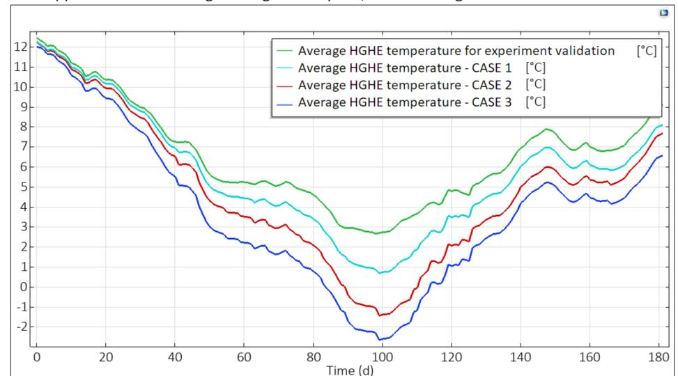
Figure 4 – Average HGHE temperature for experimental case and three simulated cases
