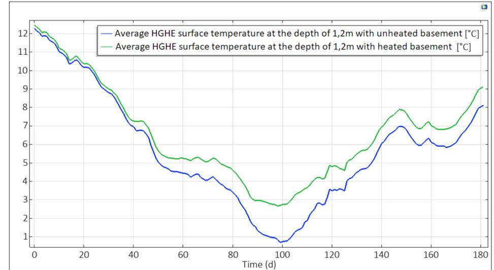
Figure 3 – Average HGHE temperature for the experimental case and unheated basement
