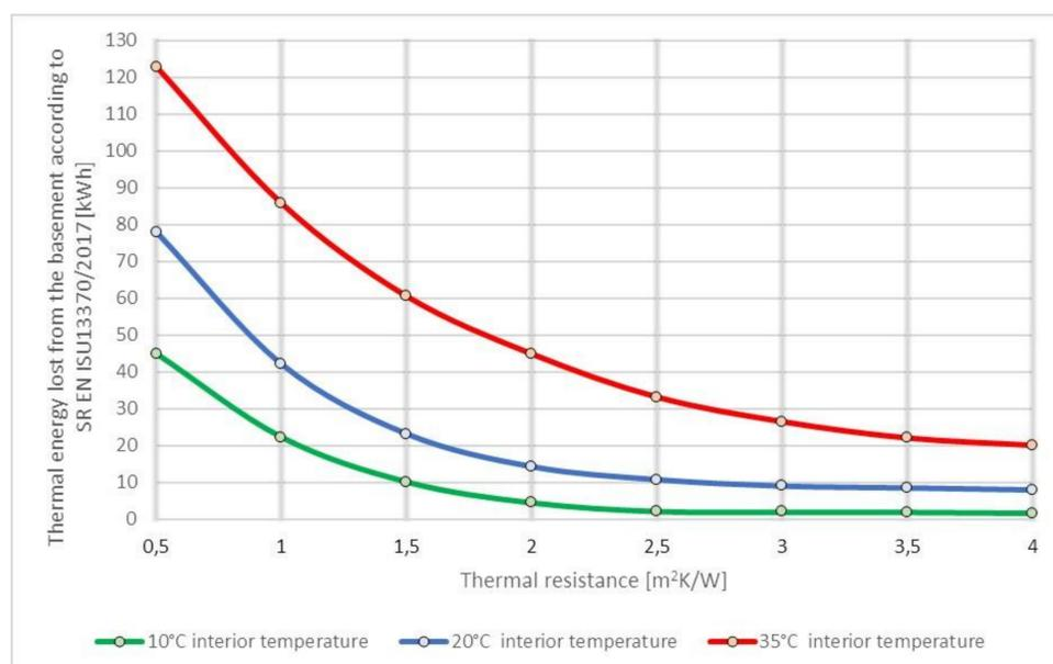
Figure 2 – Thermal energy lost from the basement to the surroundings
