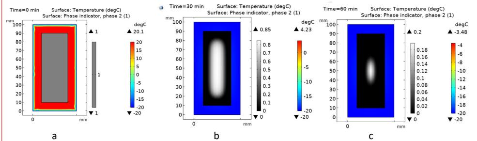
Figures 4 – Phase change indicator and temperature of the reactor at the beginning (a), after 30 min (b) and after 60 min (c)
