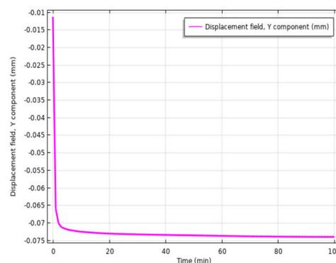
Figure 5 – Total displacement of the superior part of the reactor on Y direction [mm]
