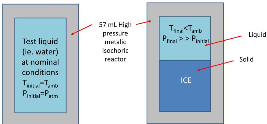
Figure 1 – Nominal conditions (left) and expected behavior inside the reactor when the isochoric reactor is immersed in a cooling bath at a negative temperature (right)
