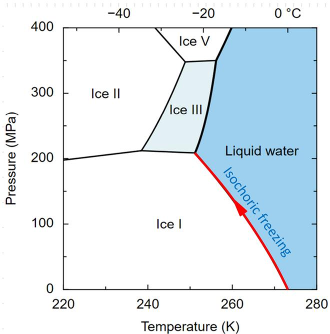
Figure 2 – Isochoric freezing processes on the phase change diagram of water
