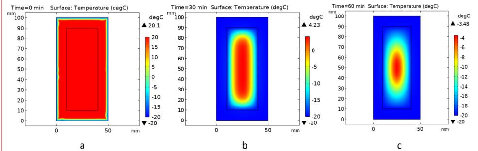
Figures 3 – Heat transfer in solid and liquid at the beginning (a), after 30 min (b) and after 60 min (c)
