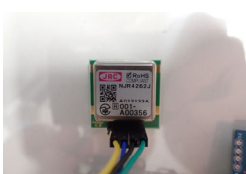
Figure 1. Microwave Doppler sensor
