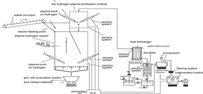
Fig. 1. The schematic diagram of equipment for hydrogen plasma conversion of construction waste
