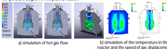
Fig. 2. Modeling and simulation of the main reactor with plasma on hydrogen
