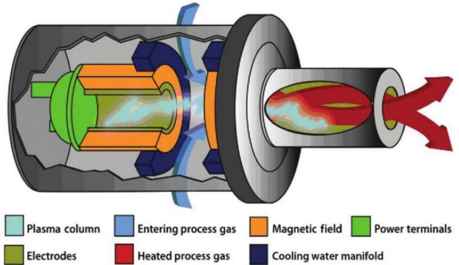
Figure 1. Plasma torch schematic.
