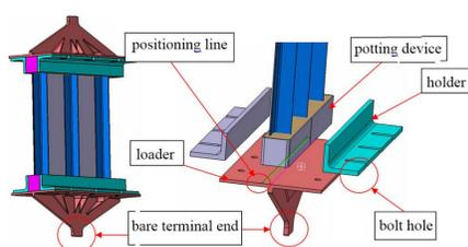
Fig.3 Schematic Diagram of test fixture
