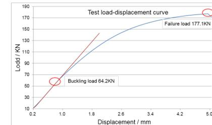
Fig.8 Test analysis-load-displacement curve
