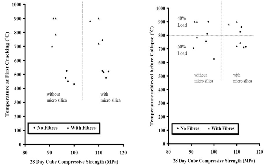
Figure 2 Temperature at first cracking and collapse temperature (unreinforced columns).
