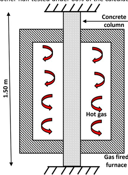
Figure 1 Experimental set-up for fire testing of high strength concrete
