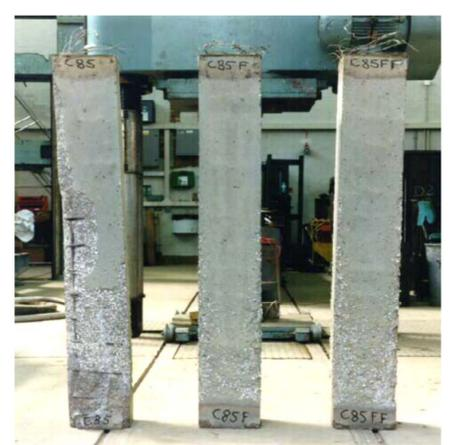
Figure 4 Comparison of C85 test specimens after test (no fibres on left, 3kg/m<sup>3</sup> p/p fibres in middle and 6kg/m<sup>3</sup> p/p fibres on right).
