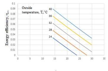
Figure 4. Exergy efficiency as a function of the heat carrier temperature for isothermal processes (a), and for non-isothermal processes (b) in case of heating.
