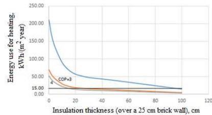
Figure 3. A heat pump supplying a 20...30 cm insulated house needs almost the same energy for heating as a passive house.
