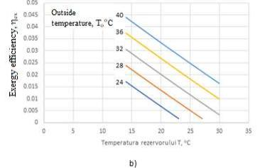
Figure 5. Exergy efficiency as a function of the heat carrier temperature for isothermal processes (a), and for non-isothermal processes (b) in case of cooling.
