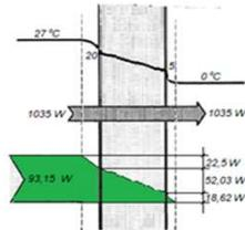
Figure 1. The flow diagram for the energy (a) and for the exergy (b).
