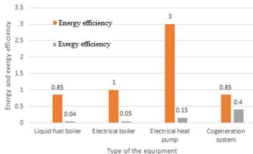
Figure 2. A comparison of the energy and exergy efficiency for some heating systems.
