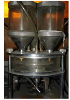
Figure4 Plasma spraying powder feeder diagram
