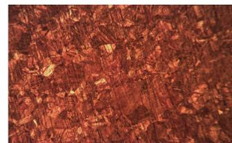
Figure5 Spiral mother QSN7-0.2 annealed metallographic structure
