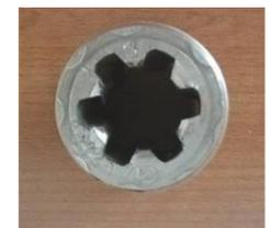
Figure6 Copper screw after thermal spraying
