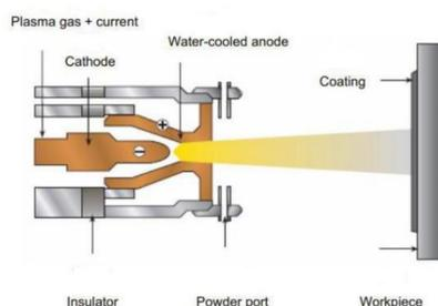
Figure2 Diagram of plasma spraying
