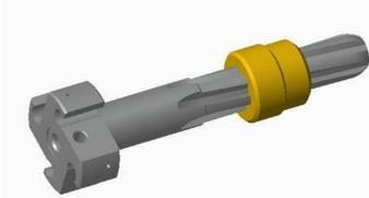
Figure1 Copper nut friction pair
